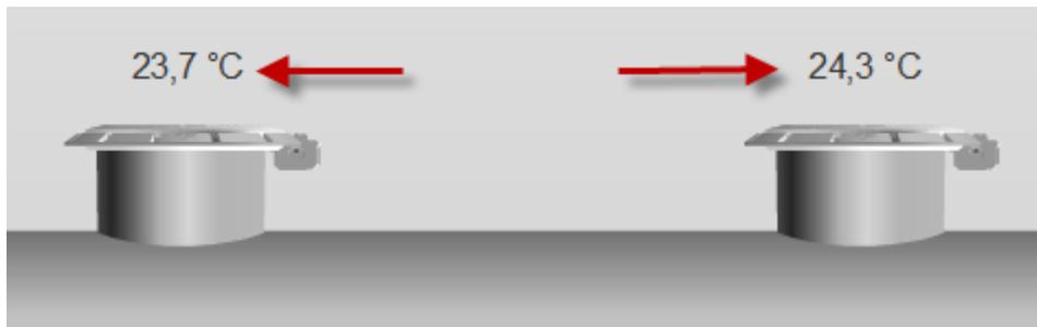
It can be used to evaluate the degree of sunstroke suffered by the caps. So if you notice very different temperatures, imply a greater degree of heating due to its positioning in the Station (for example, sun exposure, or within the coverage area).
